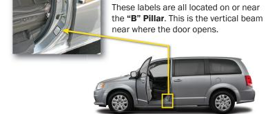
The Tire Placard label (required) is typically found on the "B" Pillar
